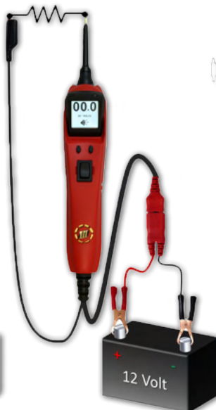
Continuity (less than 20k \Omega but greater than approx. 650 \Omega )
